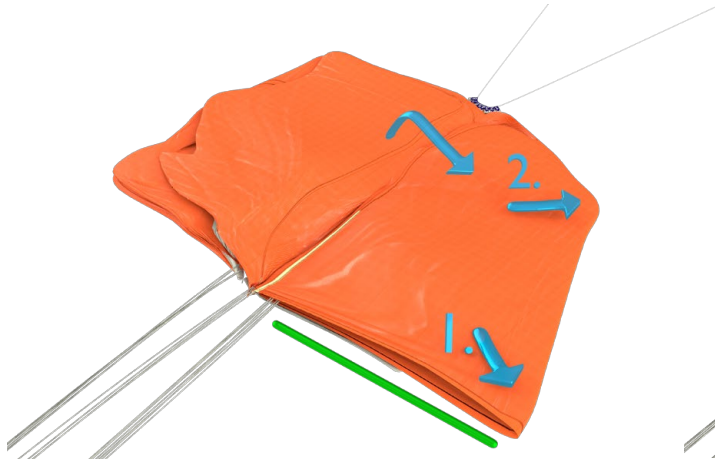
Picture 10 - Pulling out bottom and top corner.
