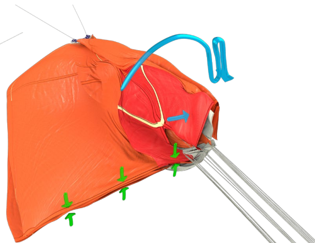
Picture 18 - Rotating s-fold under.
