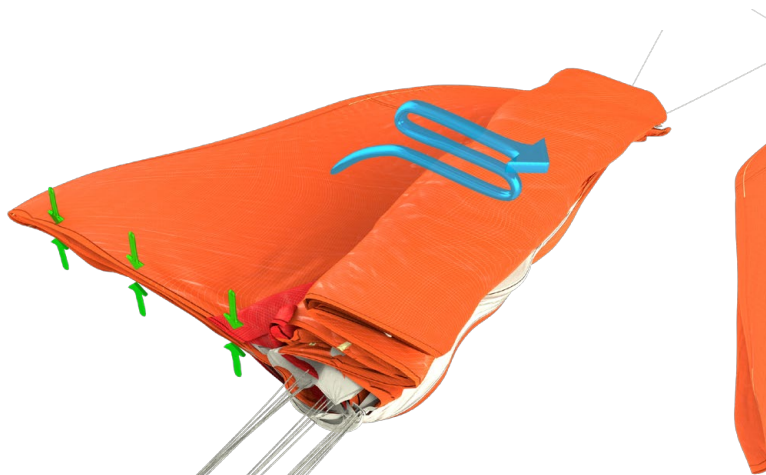
Picture 17 - S-folding lower half on top.
