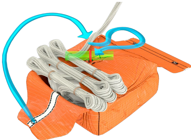
Picture 26 - Bundles inside, ready for final cover.
